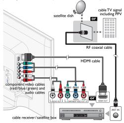
You can also connect this unit to the cable receiver or satellite box other than the HDMI or the Component Video output jacks or Composite Video output jack (**\*\*\* p.25, 26**) because they might have different output jacks.
